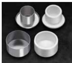
Figure 4.14 - Q600 Sample Pans (platinum pans on the left, ceramic cups on the right)
