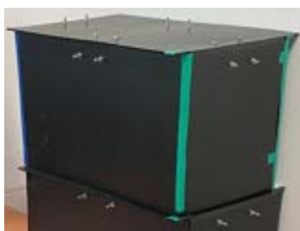
Fig. 3.3: Shading system built with plastic corrugated boards and 3M tape (Lorenzo Massimo Toniolo)
