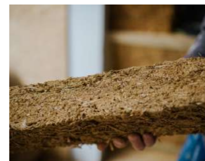
Figure St07: Non-structural straw-clay blocks Source: https://www.hgmatthews.com/lime-and-cob/natural-building-blocks/
