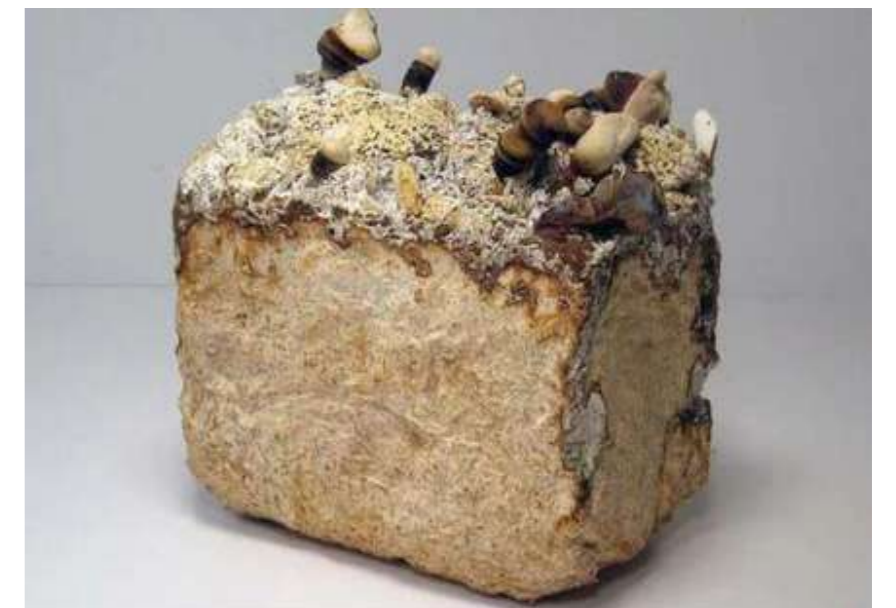
Figure 03.1.2: Philip Ross Molds Fast-Growing Fungi Into Mushroom Building Bricks, these bricks are biodegradable Source: https://inhabitat.com
