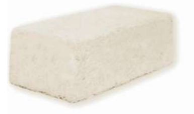
Figure My07: Mycelium brick - Grow Bio Source: https://www.grown.bio/
