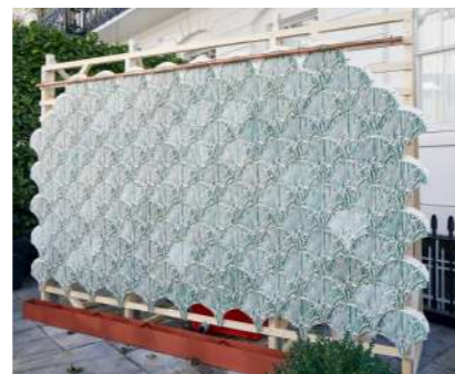
Figure Sw14: INDUS - Purifying clay-algae tiles - wall system Source: https://www.dezeen.com
