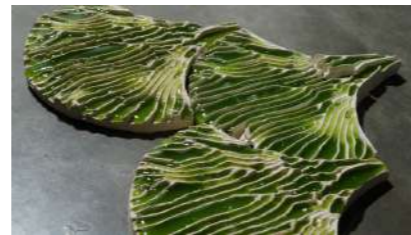
Figure Sw13: INDUS - Purifying clay-algae tiles Source: https://www.dezeen.com
