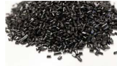
Figure Bp04: Lignin based bio-plastic pellets by the Swedish company RenCom Source: https://www.plasticfree-world.com/
