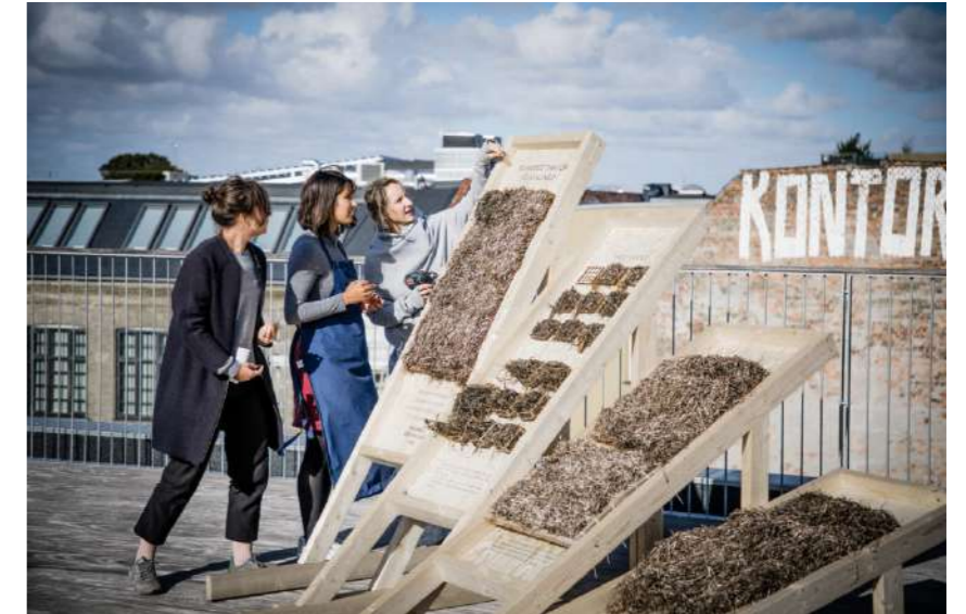
Figure Sw08: Prefabricated thatched seaweed panels by Kathryn Larsen Source: https://kathrynlarsen.com/
