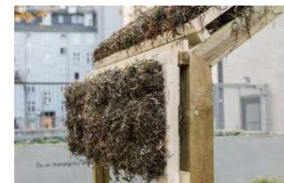
Figure Sw09: Test panel with different bio-based binders Source: https://kathrynlarsen.com/
