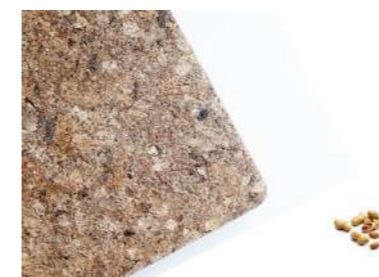
Figure Hk11: Peanut shell panel Source: https://materialdistrict.com
