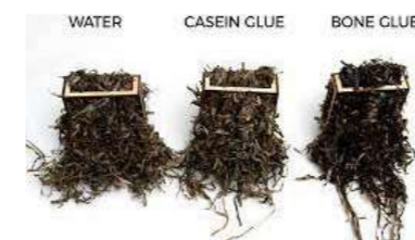
Figure Sw09: Test panel with different bio-based binders Source: https://kathrynlarsen.com/
