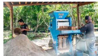
Figure Sw19: Machine designed to make adobe blocks and adjusted to make Sargablock
