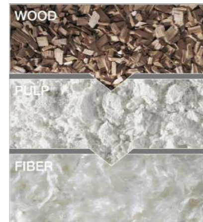
Figure Cp01: From wood to cellulose fibre
