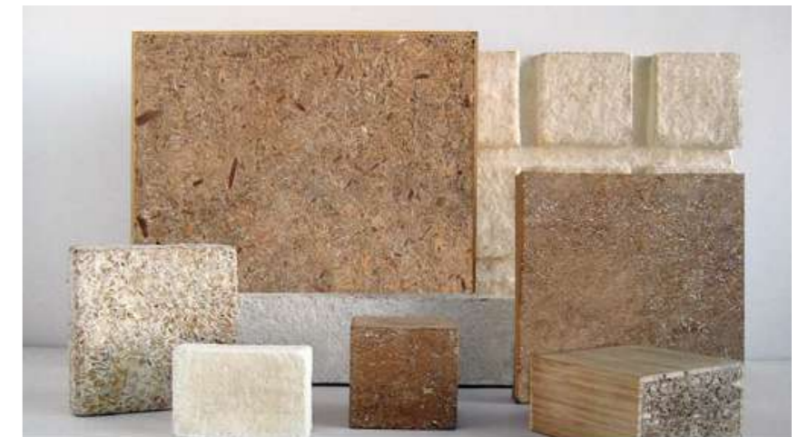
Figure My10: Mycelium panels Source: https://www.researchgate.net/figure/Various-mycelium-based-panel-product-samples-Image-supplied-by-Phil-Ross_fig2_361056782
