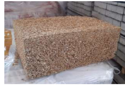
Figure Hk12: Rice husk brick - by Rice House Source: https://materialdistrict.com/article/a-house-made-of-rice/
