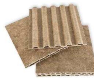
Figure Pf16: Hemp panels by Jory Swart Source: https://theexplodedview.com/materialbb/hemp-panels/
