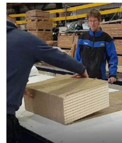
Figure Pf23: Composite blocks that compose the main structure of the bridge made from foam core wrapped with flax fibre Source: https://www.dezeen.com/2022/05/05/smart-circular-bridge-flax-completed-the-netherlands-architecture/
