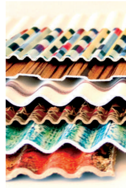
Figure Cp07-08: Wellboard - cellulose fibre board - by Kraftplex Source: https://materialdistrict.com/material/wellboard/
