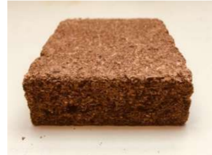
Figure Ms02: Peat moss panel bound with tannin-based adhesive Source: Morandini, M. C., Kain, G., Eckardt, J., Petutschnigg, A., & Tippner, J. (2022). Physical-Mechanical Properties of Peat Moss (Sphagnum) Insulation Panels with Bio-Based Adhesives. Materials , 15(9), 3299. MDPI AG. Retrieved from http://dx.doi.org/10.3390/ma15093299
