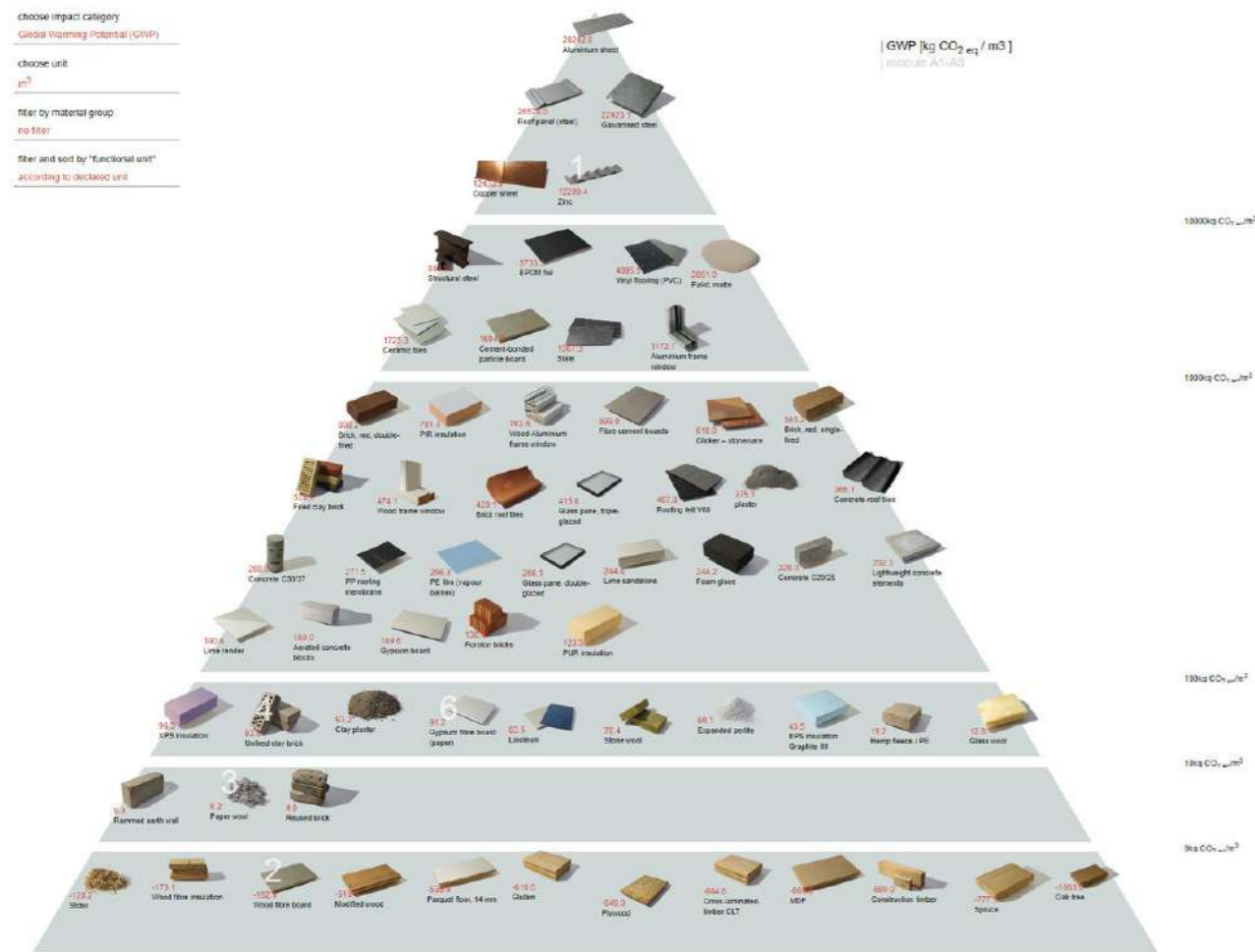
Figure 01.3.4: Pyramid of environmental impact of building materials expressed in GWP Source: Developed by the Royal Danish Academy Centre for Industrialized Architecture (Cinark) developed the Construction Material Pyramid
