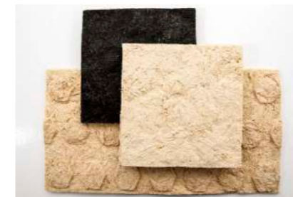
Figure Hk07: // Cornspan Corn husk panels - by Apilada Vorachart Source: https://materialdistrict.com/material/cornspan/
