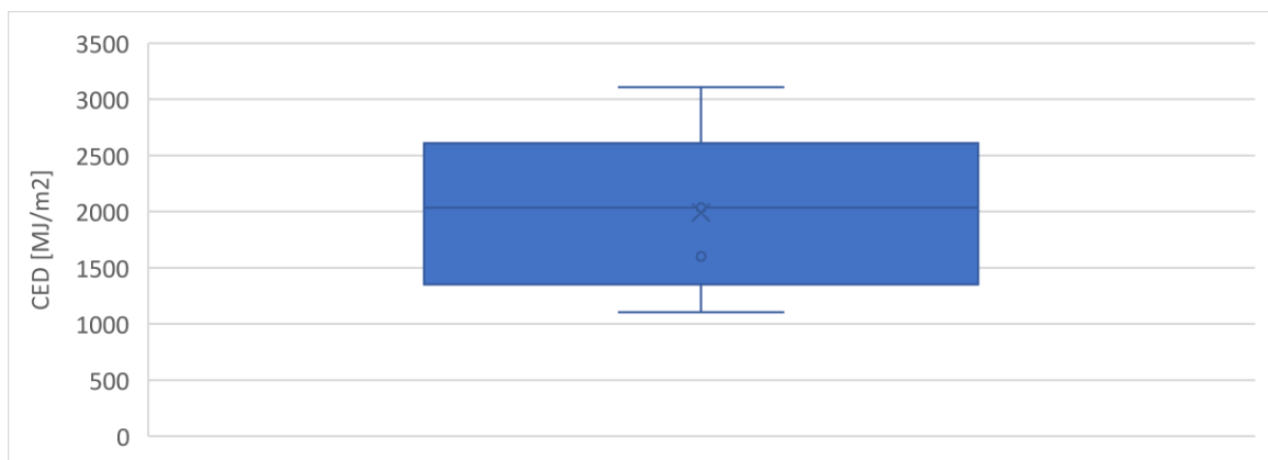
Figure 36: Values encountered in the literature for the cumulative energy demand for CIS modules manufacturing (Own production).
