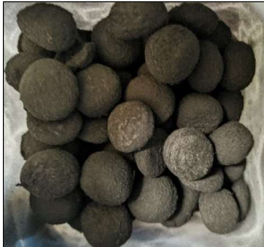
Figure 3.6 SABC produced by steam activation of the pellets.
