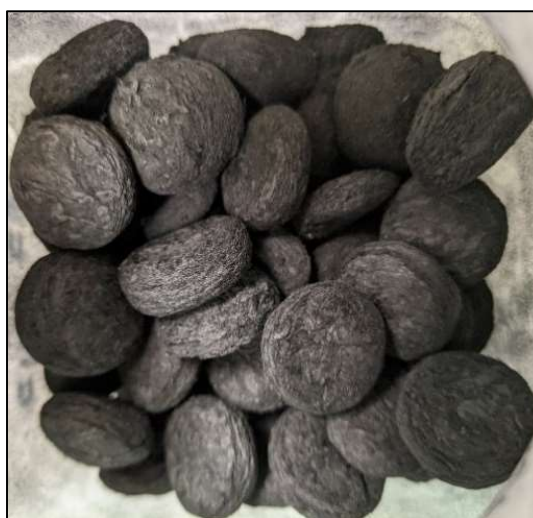
Figure 3.4 BC obtained after the pyrolysis of the recycled textiles pellets
