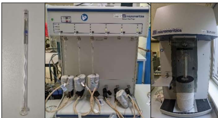
Figure 3.8 BET quartz glass tube (on the left), vacuum degassing unit (in the middle) and Micromeritics 3Flex unit for surface area determination (on the right)
