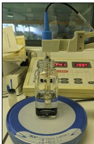
Figure 3.10 pH meter used for the measurement of the pH point of zero charge.
