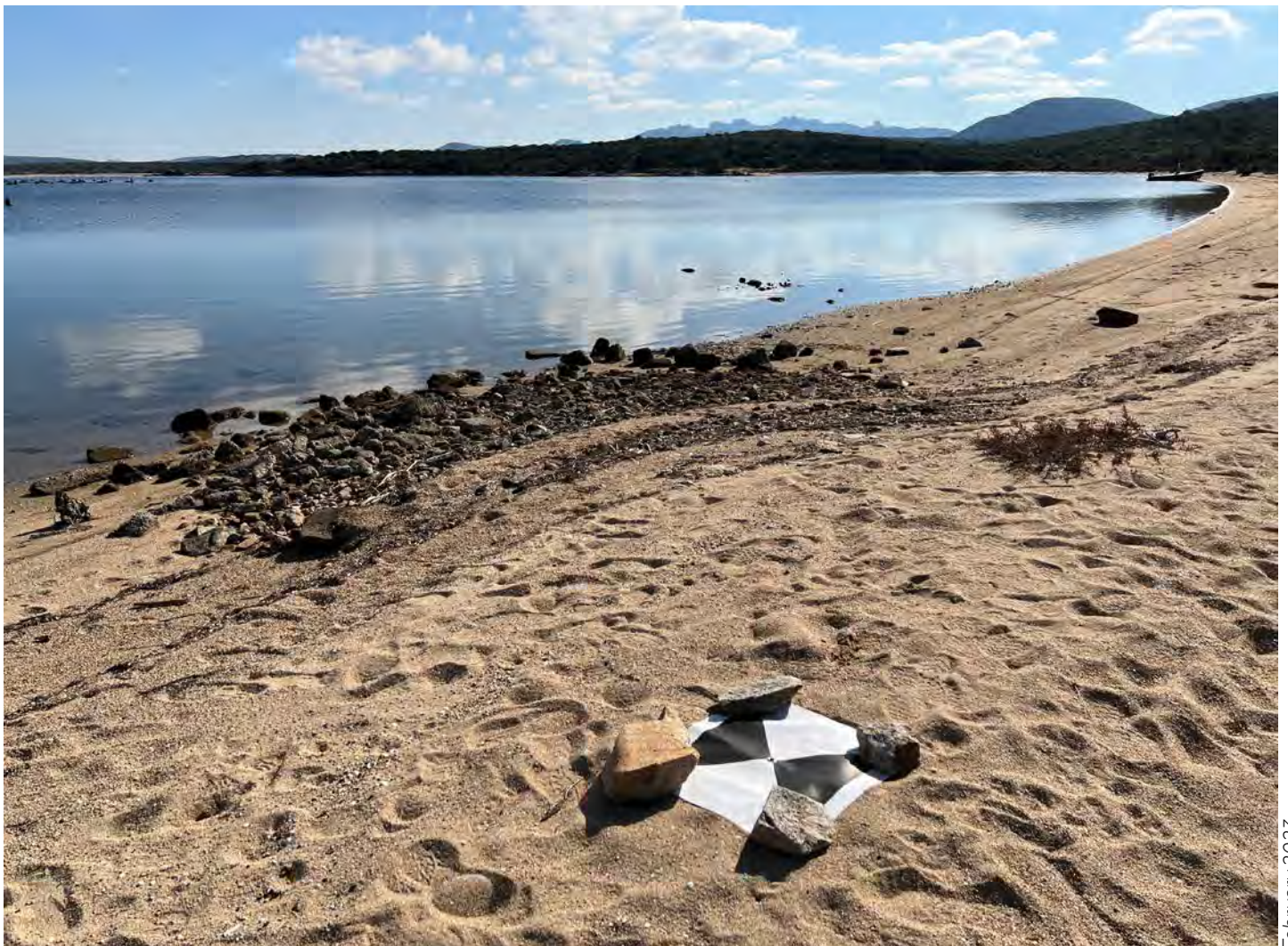
"Targeted" GCP marker measured with the rover
