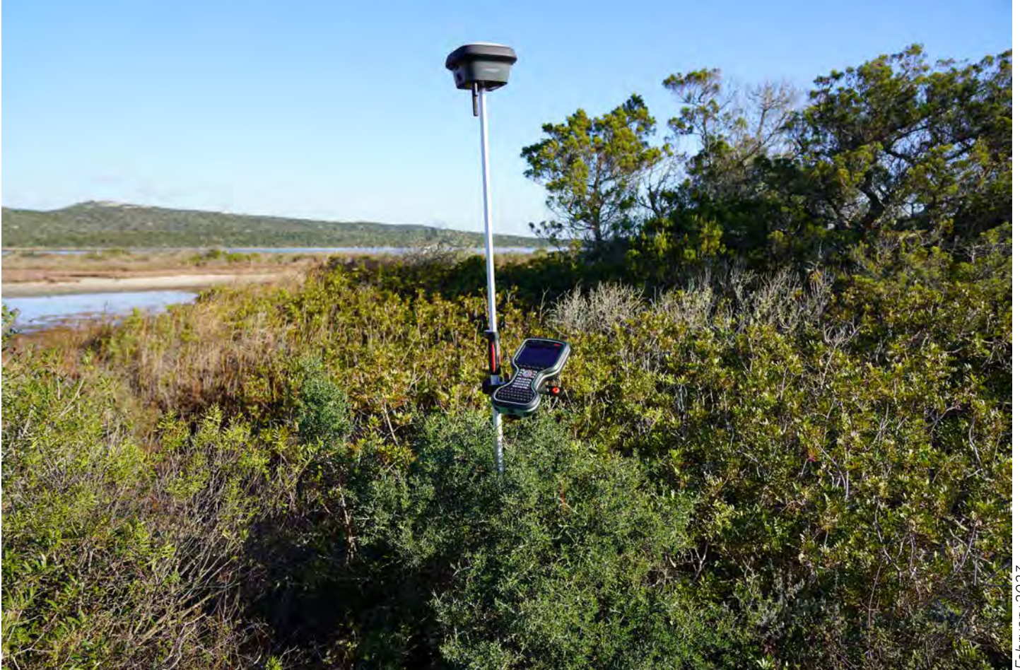
"Leica CS20 Field Controller" (below) e "Leica GS18 GNSS RTK Rover" (above) with tilt error correction technology 7 - geolocating plant species
