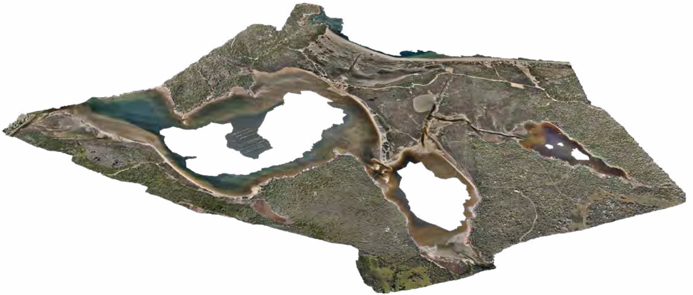
Entire 3D model as a triangulated and interpolated mesh
