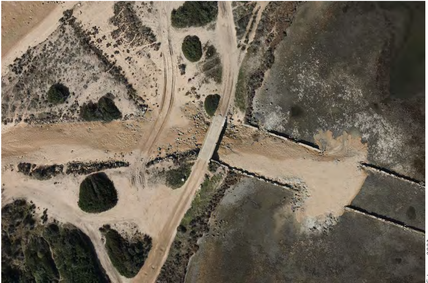
Current traces of the concrete bridge, canal, and triangular fishing system of "Bocche Gauliane" designed to be overflooded with high tide
