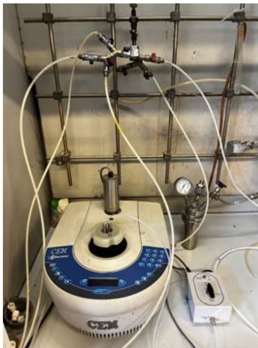
Figure 24. CEM modified microwave with external pressure control system.
