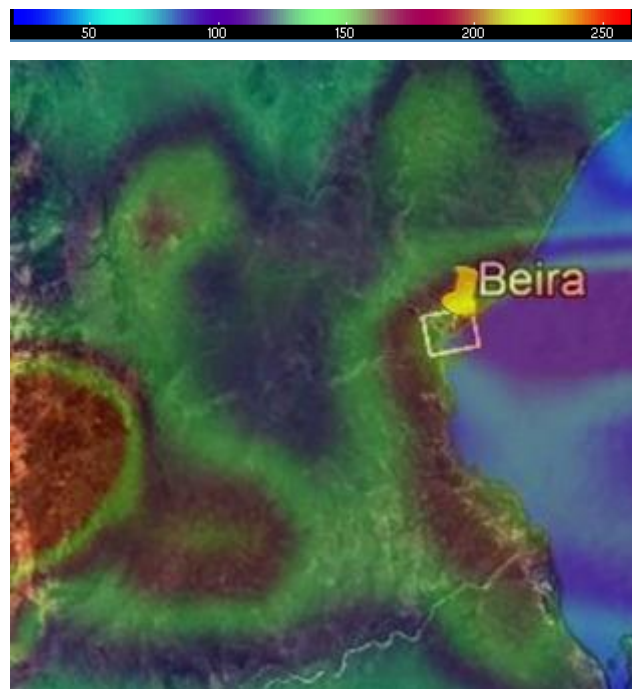
Figure 18: Representation of the values of Rx1day computed starting from reanalysis data, for the year 2019 over the area of interest. This image demonstrates that the index of extreme rainfall contains information about the criticality of that year for Beira, given the high values reported (reddish areas). From this point, an empirical approach described in this paragraph was developed to construct a criterion whereby, starting from indices values, one year is defined as “critical” for Beira.
